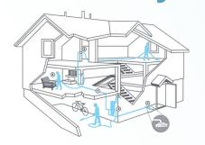
of the contacted dirt, dust and allergens away from living area to the central power unit located in the garage, and is the only central vacuum recommended by the NZ Asthma Foundation
